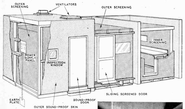
also be seen the two rails on which the doors run, the tapered coppercovered floor ramp, and the contact springs on the leading edge of the doors. There is also an outer hinged door to complete the acoustic screening.
