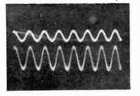
Fig. 15. Oscillogram of the output (top) and the input (bottom) at 1,000 c/s. both tone controls set to minimum.
