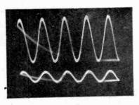
Fig. 14. Oscillogram of the output (top) and input (bottom) at 10,000 c/s. with the treble tone control at maximum and the bass tone control at minimum.
