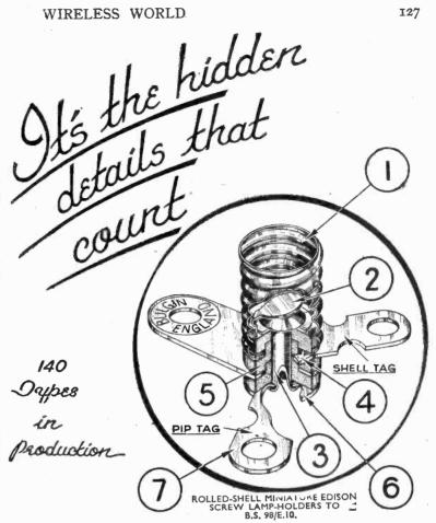
Threaded shell with dimensions and details to B.S. 98—10 mm. "MES"; silver-plated finish.
