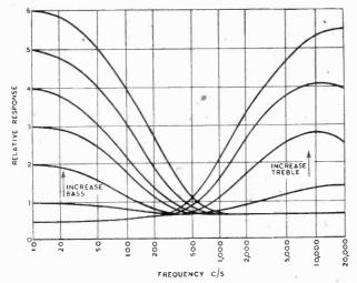
Fig. 13. Experimental results obtained from the circuit as shown in Fig. 12, omitting condensers  $C_5$  and  $C_7$ . The "increase bass" readings were taken with the treble tone control at minimum and the "increase treble" readings with the bass tone control at minimum.
