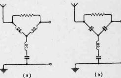
$\mu$ H coil, and wish to reject a frequency of 798 kc/s ( $\omega = 5 \times 10^6$ ), we find that R = 250Q ohms.
