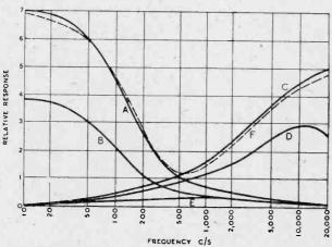
Fig. 17. Measured characteristics of the circuit as shown in Fig. 12 with  $C_5=$  0.01  $\mu F$  and  $C_7=$  0.003  $\mu F$ .
