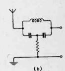
Fig. 2. Centre-tapped rejector circuits with "cancellation resistance"
