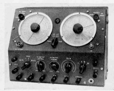
Labgear "Electronic Fault Tracer" for general testing and service work.
