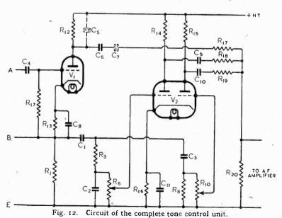
$V_{1-6C5}$  uF.  $V_{1-6C5}$ .  $V_{2-6N7}$  (or two single triodes, e.g., 6C5's.)  $R_{16}^{17}$  = 100,000  $\Omega$ .  $R_{19}$  = 100,000  $\Omega$ .  $R_{20}$  = 1  $M\Omega$ . The numbering of these components is the same as that used in the basic circuits.
