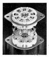
Top and bottom views of "Clix" type BoG valve-holder for all-glass valves. The sockets are anchored to minimise the risk of flash-over between pins or breakage through misalignment.
