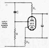
Fig. 1. Circuit suitable for fixed load
