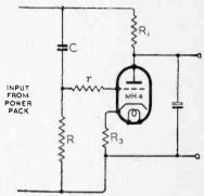
Fig. 2. Circuit suitable for any value of fixed load, without further adjust-
